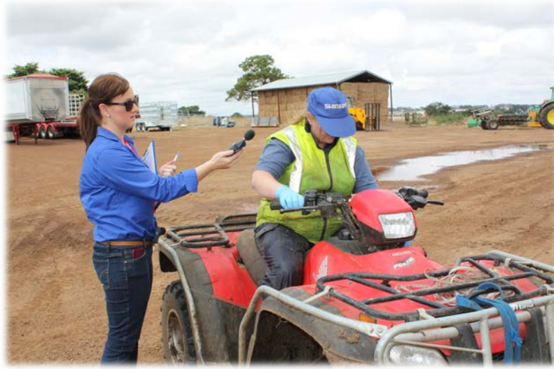
Figure 11: Testing the dB level of the Quad bike. Please note: a helmet was recommended for useage.
