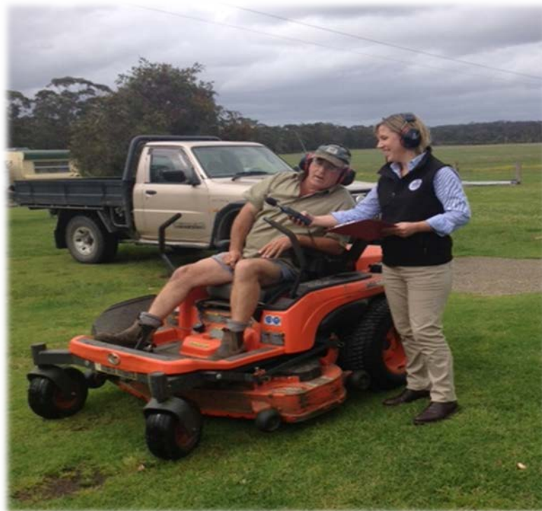
Figure 3: Undertaking on-farm noise audits using the CEL-244 digital integrating Sound Level Meter, Gippsland Victoria.
