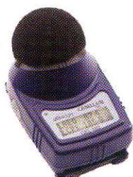
Figure 2. A noise dosimeter worn on the lapel by farmers in the Shhh hearing project.
